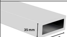
A 3D perspective view of a rectangular aluminum profile. The height is labeled as 35 mm and the width as 55 mm. | PERFIL RECTANGULAR<br>55 x 35 | 001096     |
